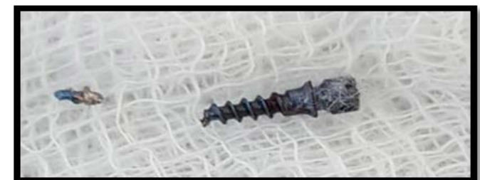
Fig 4: Fractured fragment and the total length of screw.
