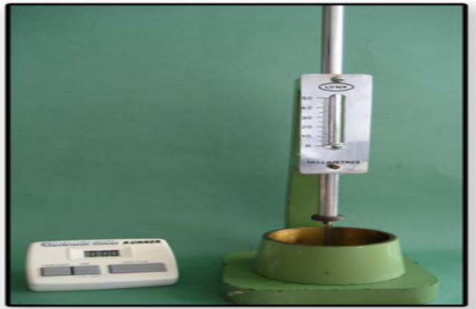
Figure 2 : Needle penetrometer and digital timer/ stop clock
