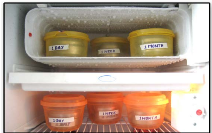
Figure 4 : Storage of PMMA resin at dough stage in deep and normal freezers
