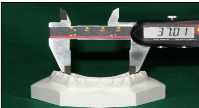
Fig 1: Arch width measurement taken from cusp tips to cusp tips of canine, premolar and first molar with digital caliper
