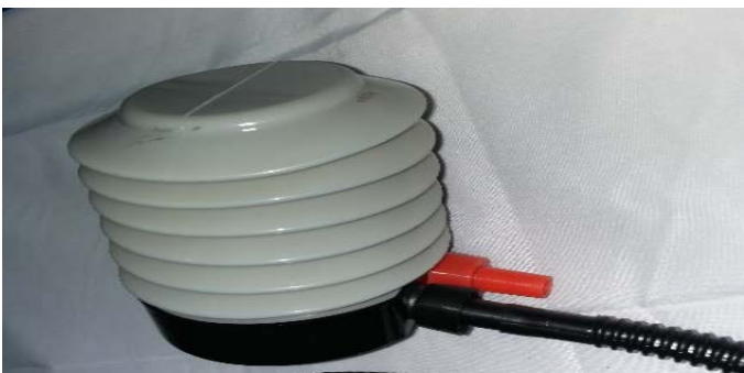
Fig.6.d Manual Hand air pump (with air in-let & out-let)
